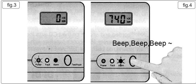
NOTE: Test this alarm when the "ppm" symbol is displayed in the LCD after the batteries have been installed. Though this alarm can self-diagnose the amplifying circuit and sensor, it is recommended that you test your CO alarm once a month to ensure it is working correctly.
